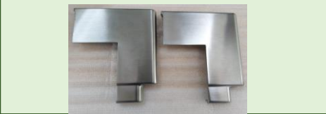
5.5 Hard Chrome coating on Steel
