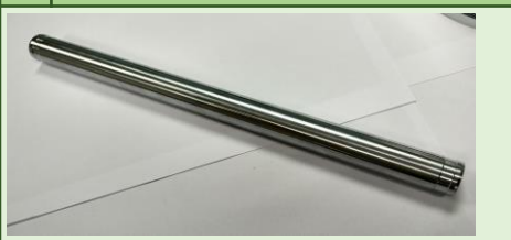
5.5 Hard Chrome coating on Steel
