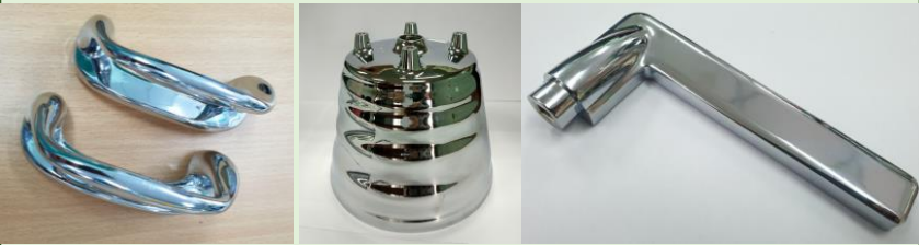
5.3 Cu-Ni-Cr coatings on Zinc with Hairline
